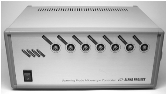
Fig. 3 Photograph of the SPM controller. Height: 133mm, width: 320mm, depth: 230 mm.
